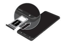
4. Slide the SIM card/Memory card tray back into the slot.
