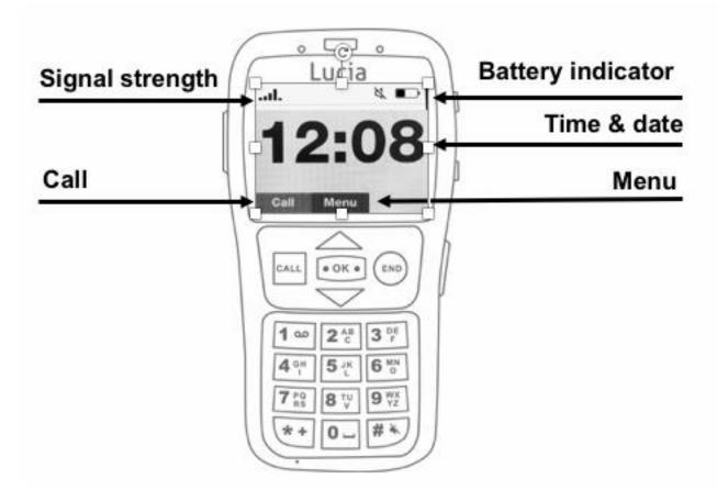
The home screen has several icons arranged around the screen. Top left is the signal strength indicator and wireless provider name. In the center there are indicators as per the overview shown below. On the right is the battery indicator. The battery icon will indicate the remaining battery charge level.
