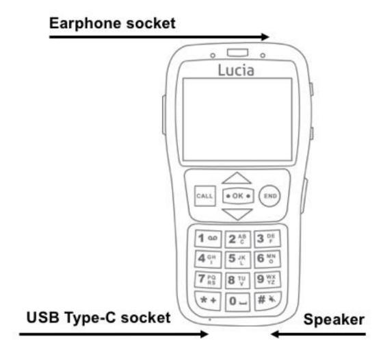
On the top edge, near the right end of the phone there is a small round hole which is the earphone socket. It is a standard socket for a 3.5 mm audio jack.
