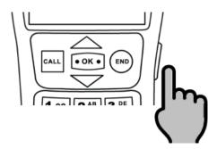
When the phone isn't used for a period of time, the keypad lock is automatically activated. You can unlock the keypad by briefly sliding up the **Lock/Unlock & Power button/slider** located on the right edge of the phone.
