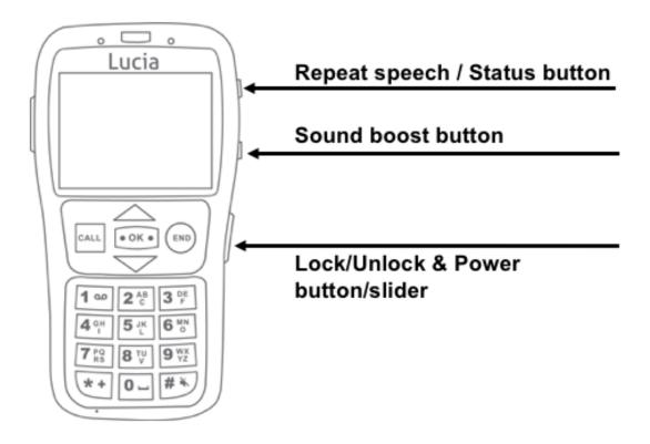
There are three buttons on this edge. From top to bottom they are the following: **Status/Repeat speech button** and then the **Sound boost button**, followed by the **Lock/Unlock & Power button/slider**. The Repeat speech button serves as the phone **Status button** and can be used to turn the Voice guide ON or OFF as well (press and hold).
