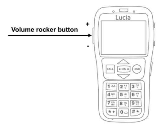
On the left edge, near the top of the phone is the **volume rocker button** with up at the top and down underneath.
