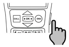
To turn off the phone, ensure the keypad lock is not active and that you are at the home screen. Slide the slider up and keep it in this position for at least 3 seconds until you hear a prompt that the phone is turning off.
