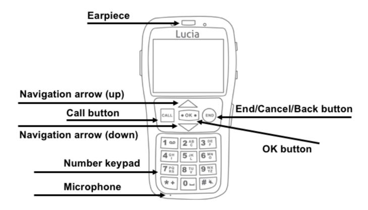
The front face of the phone has five buttons underneath the screen. On the left is the square green **Call Button**, on the right is the round red **End/Cancel/Back button**. Between these buttons are the **up/down navigation** arrows. Between the navigation arrows is the rectangular blue **OK button**.
