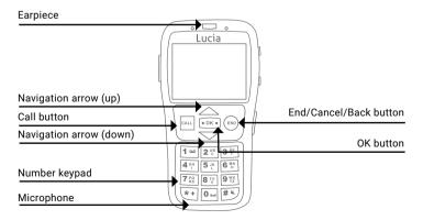
The front face of the phone has five buttons underneath the screen. On the left is the square CALL button (green) and on the right is the round END/Cancel button (red). Between these buttons are the up/down navigation buttons. Between the navigation arrows is the smaller, rectangular OK button (blue).
